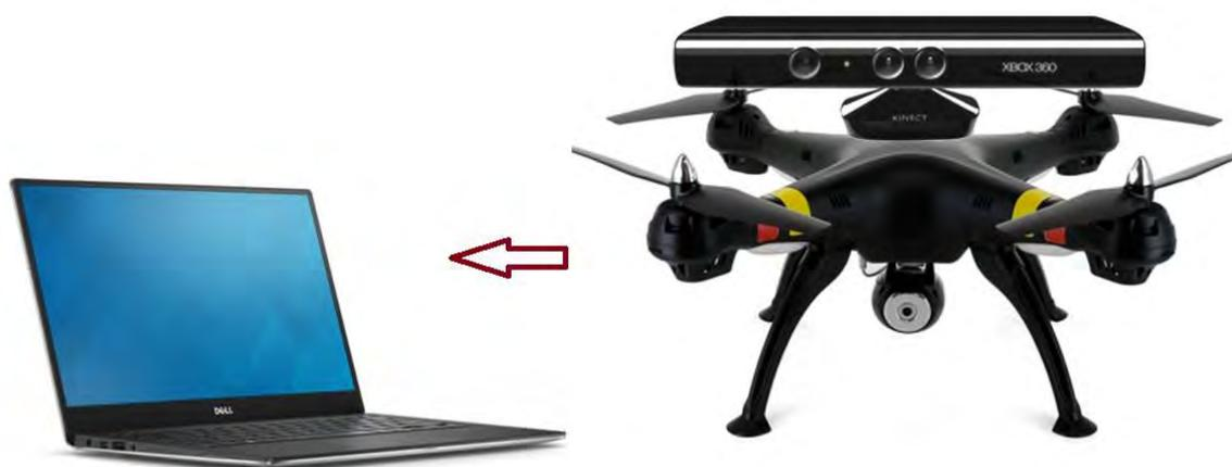
Fig. 3.7: Shows the Kinect mounted on top of the quadcopter and connected to the workstation
